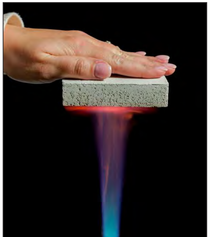
Pratliperl Concrete is Fireproof and has a low Thermal Conductivity Typical k=0.13 \text{ W/m}^\circ\text{C}
