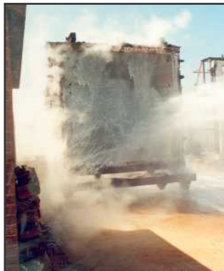
Hose stream application after one minute.
